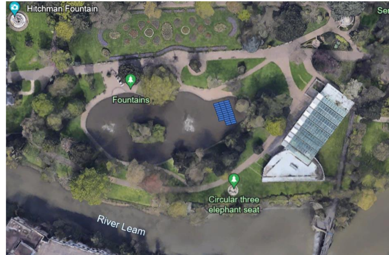
Water Source Heat Pump Array. Kensa 2023
