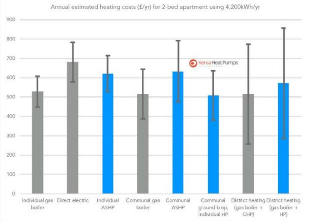
Comparison of predicted heating costs for the resident(s) of a 2-bed energy efficient apartment
