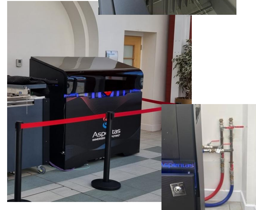
Exemplar Demonstrator – Immersion cooled by running in a tank of dielectric fluid
