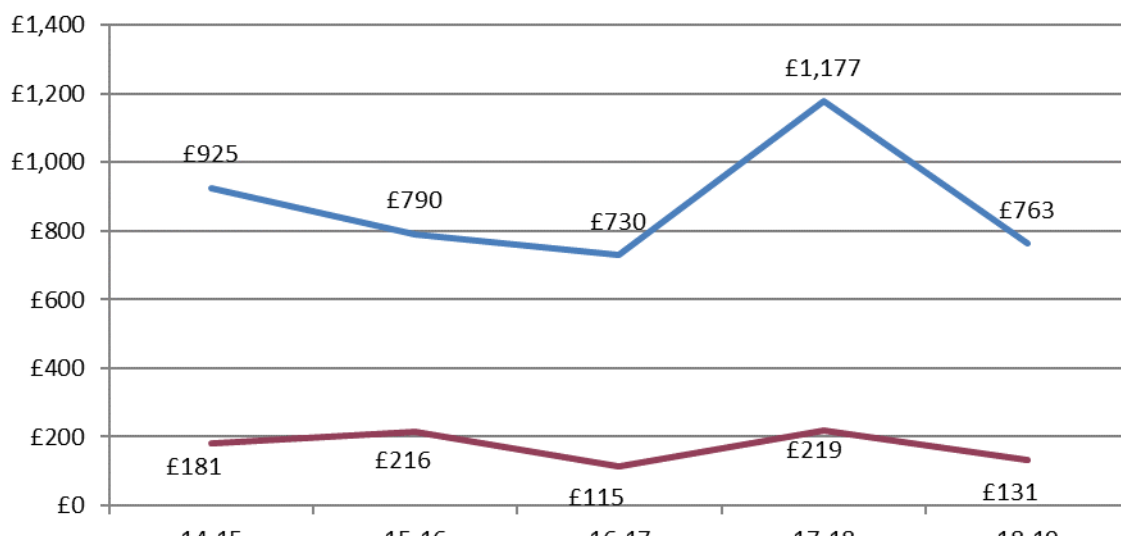
PI 50 Total cost for footway winter maintenance treatment over the entire winter period divided by the total footway network length PI 43 Total cost for carriageway winter maintenance treatment over entire winter period divided by the total carriageway network length
